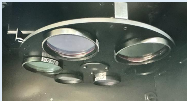
Six position filter wheels with emission filter
