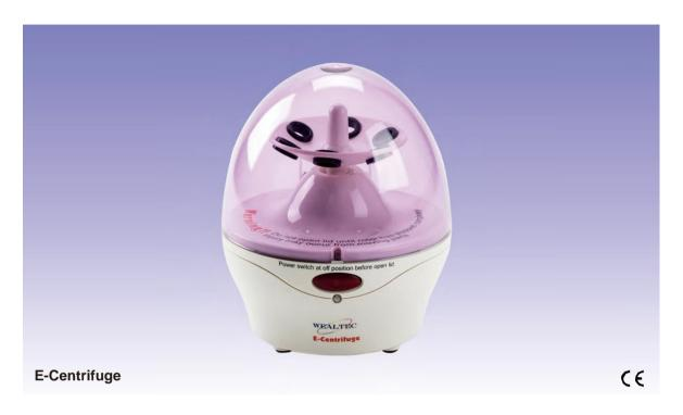
Small footprint desktop centrifuge is designed for quick spin down from the suspension. Supply with interchangeable angle rotor for 6 positions of 1.5 / 2.0ml tubes, and strip rotor for 8 x 2 positions of 0.2ml PCR tubes. Optional adapter is available 0.4 / 0.5ml tubes, and interlock switch secures top lid suddenly opened.
