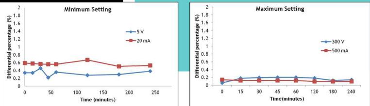
Stability of ELITE 300U with (A) minimum and (B) maximum setting.
