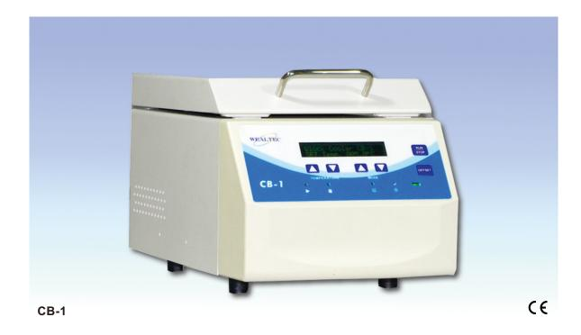
Moisture free on the bench is the main focus of Block Cooler; nine preset temperature programs satisfy different applications from  $0 - 75^{\circ}\text{C}$  with  $\pm 1/2 - 0.5^{\circ}\text{C}$  accuracy. OFFSET function is designed for self-temperature calibration, and multi-color LED is used as status indicator light; Orange-running, Redheating, Green-cooling and OK-ready to work.
