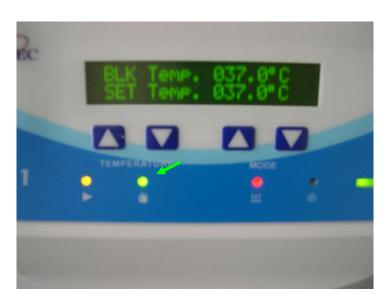
**Figure 4:** When the target temperature has been reached, as indicated by the display and the green "ready"-indicator glowing steadily (green arrow), the block cooler is ready to be used.
