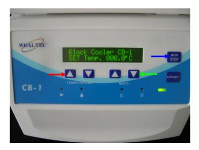
**Figure 2:** Set one of the pre-programmed temperatures by pressing on the "up/down" arrows above "MODE" (green arrow). For fine-tuning or customised temperature setting, press the "Up/down" arrows above "TEMPERATURE" (red arrow). To start heating or cooling, press the "RUN/STOP"-button (blue arrow).
