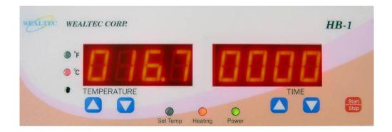
**Figure 2:** Once the block heater starts warming up, the left display will show the current temperature and the "Heating". The power indicators will be lit.
