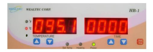
**Figure 3:** When the unit is warm enough, the "Heating" indicator will turn off. Press the Stop/Start-button to access the timer-settings. The time will be shown on the right display.
