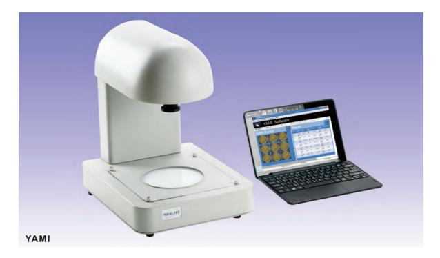
YAMI colony counter equipped with white/blue trans light source and powerful Auto-Count software offers rapid and complete solution for spiral plate, Ames, and even GFP colony. Auto counting design simplifies the routine work into one click. Batch of colony plates can be counted within minutes. Image captured by high resolution camera that even the minute different can be distinguished.
